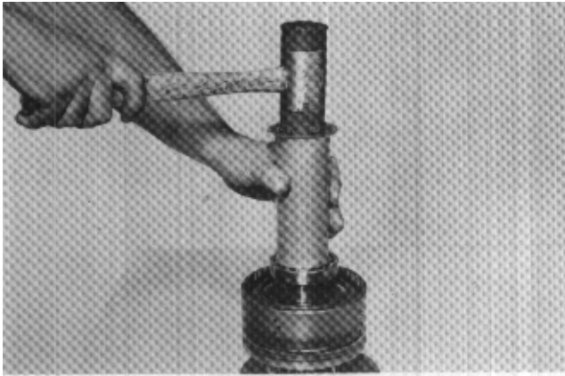
Figure 81 Install low speed gear inner bearing.
