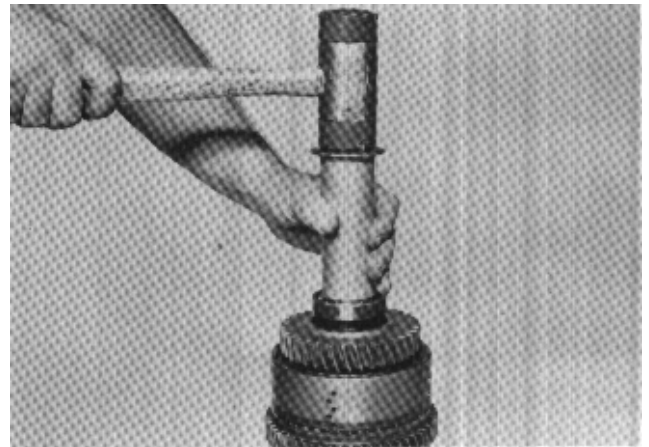
Figure 108 Install outer spacer.
