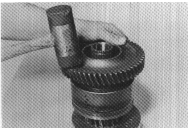
Figure 83 Install low clutch driven gear and hub into clutch drum. Align splines on clutch hub with internal teeth of friction discs. Tap gear into position. Do not force this operation. Gear splines must be in full position
