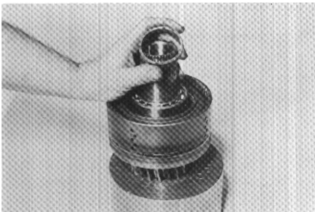
Figure 82 Install low speed gear bearing spacer.
