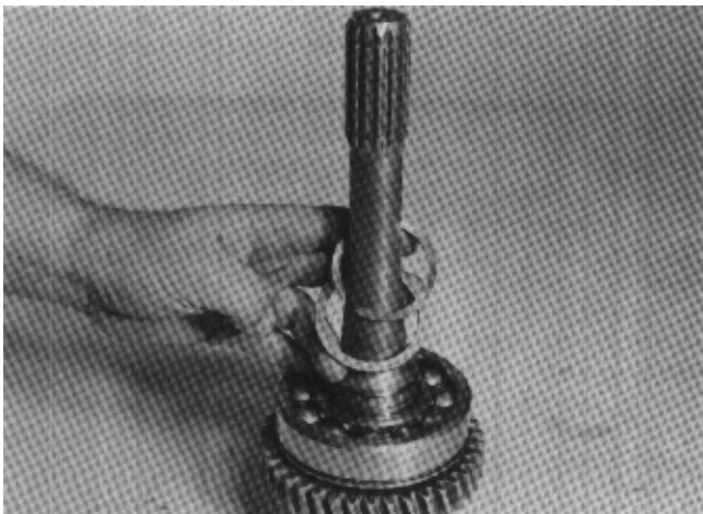
Figure 119 Remove oil sealing ring and turbine shaft bearing retainer ring and washer.
