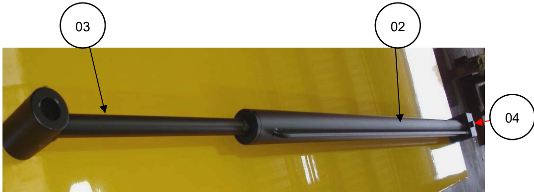
BALE CYLINDER (PIN EYE WELDED TO ROD)
