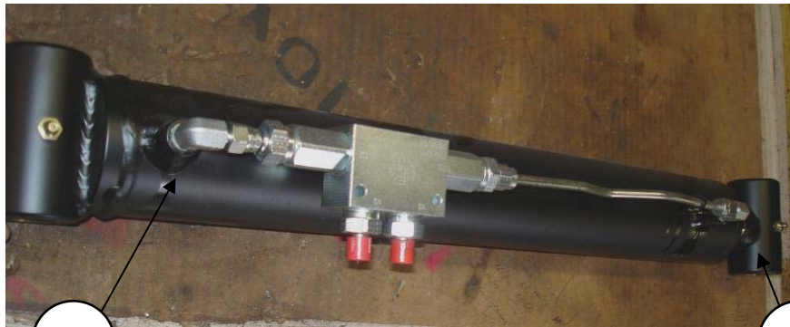
02 BALE CYLINDER (PIN EYE WELDED TO ROD) 03
